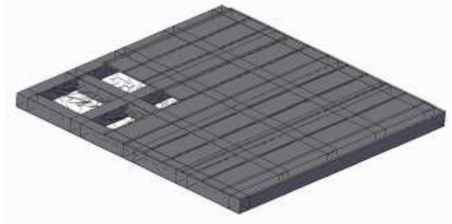
Figure.14, (b) 3D-view of wooden sheds covered with a thick wooden panel fixed with nails
